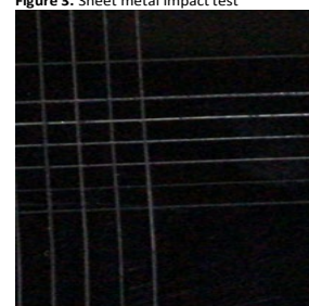
Figure 6. Sheet metal surface adhesion test
