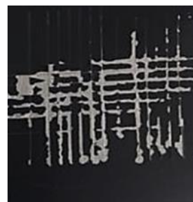
Figure 5. Galvanized surface adhesion test
