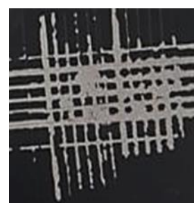
Figure 6. Sheet metal surface adhesion test
