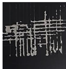
Figure 5. Galvanized surface adhesion test
