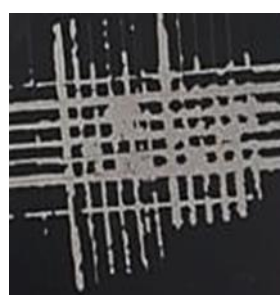
Figure 6. Sheet metal surface adhesion test
