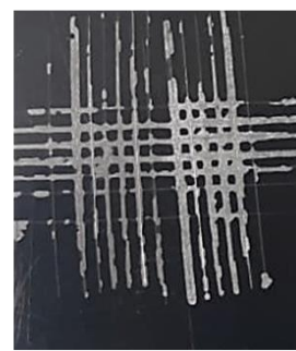
Figure6. Sheet metal surface adhesion test
