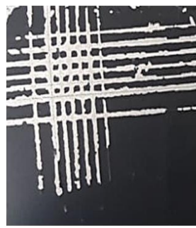
Figure5. Galvanized surface adhesion test
