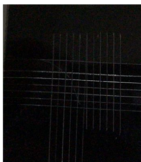
Figure 4. Aluminum surface adhesion test
