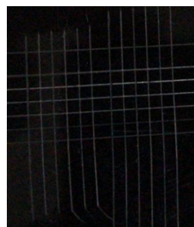
Figure 5. Galvanized surface adhesion test
