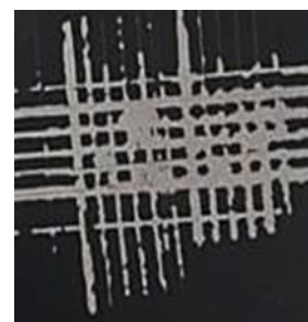
Figure 6. Sheet metal surface adhesion test
