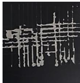
Figure 5. Galvanized surface adhesion test
