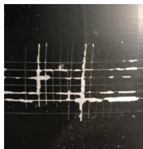
Figure 6. Sheet metal surface adhesion test
