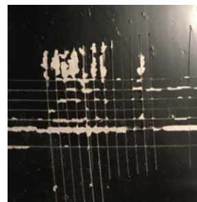
Figure 4. Aluminum surface adhesion test
