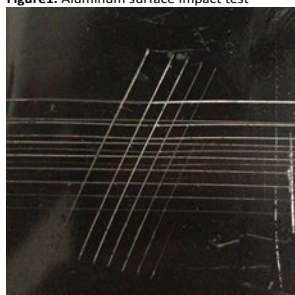
Figure 4. Aluminum surface adhesion test
