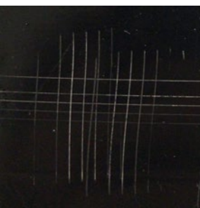
Figure 4. Aluminum surface adhesion test
