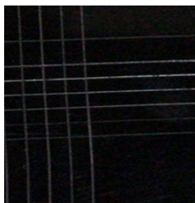
Figure 6. Sheet metal surface adhesion test
