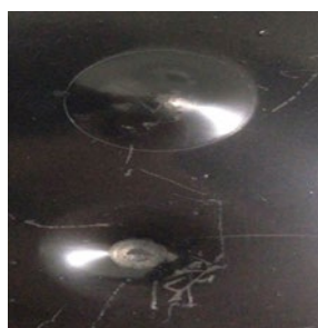
Figure 2. Galvanized surface impact test
