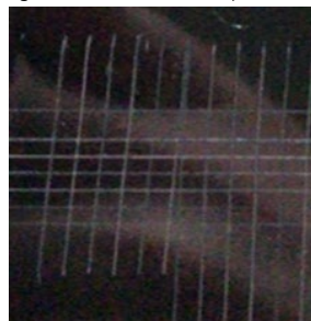
Figure 4. Aluminum surface adhesion test
