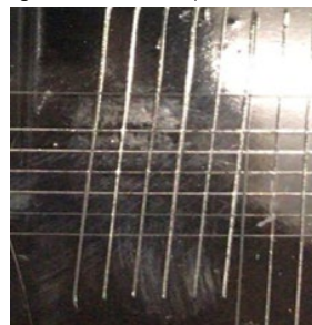
Figure 6. Sheet metal surface adhesion test
