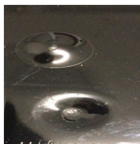
Figure 2. Galvanized surface impact test
