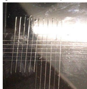
Figure 5. Galvanized surface adhesion test
