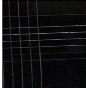
Figure 6. Sheet metal surface adhesion test
