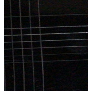
Figure 6. Sheet metal surface adhesion test
